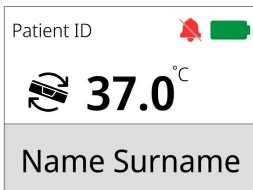
**Figure 15.34** Muted tilt alarm in a chamber
