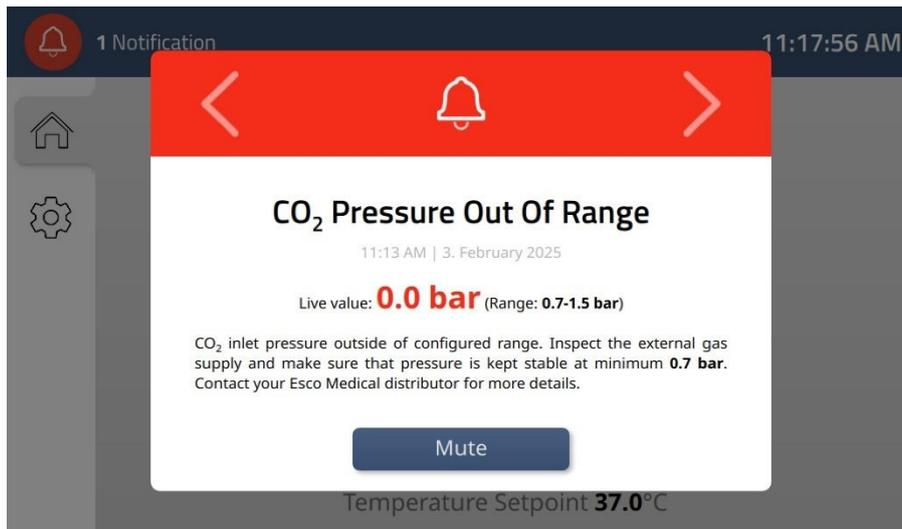
**Figure 15.17** CO<sub>2</sub> pressure out-of-range alarm indication on the docking station's display panel
