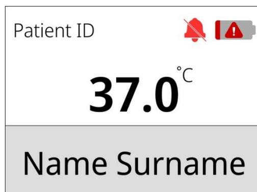
Figure 15.30 Muted critically low battery alarm
