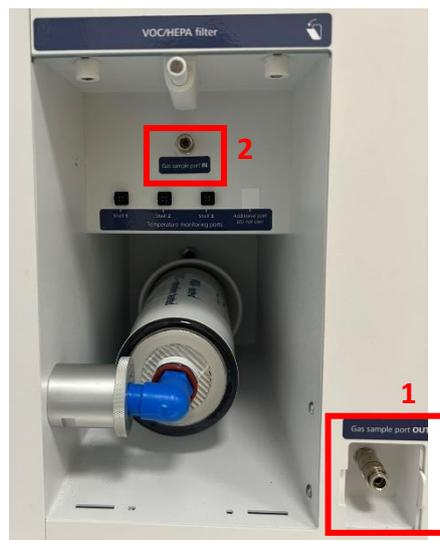
Figure 23.1 Gas sample ports
