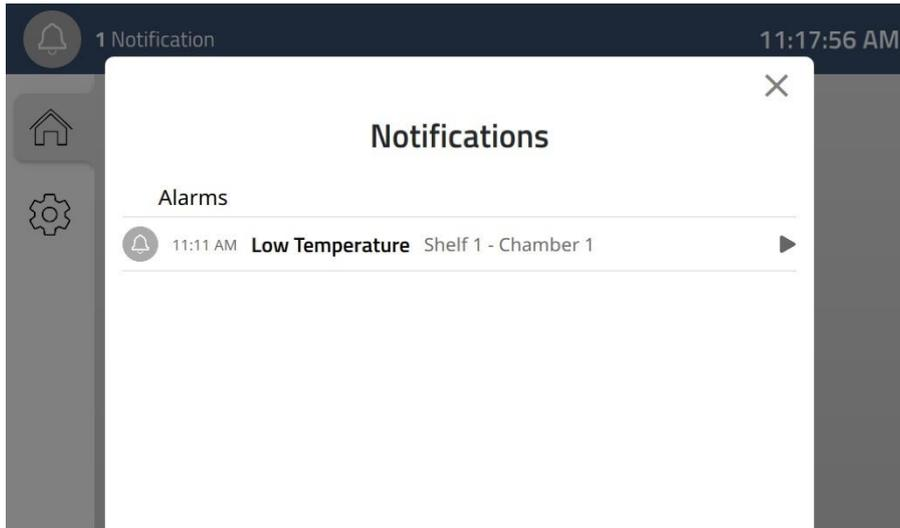
**Figure 15.42** An unacknowledged alarm in the notification list
