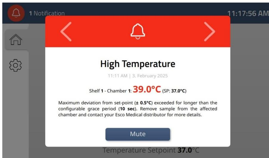
Figure 15.6 High-temperature alarm indication on the docking station's display panel
