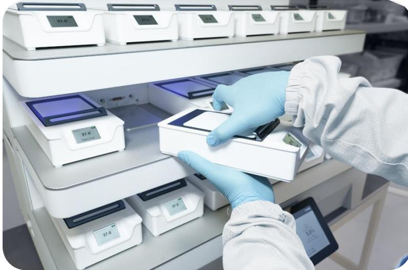
Figure 14.33 The recommended docking and undocking approach
