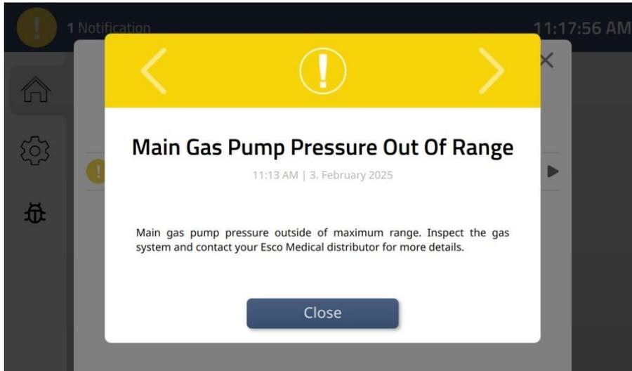
**Figure 15.52** Main gas pump pressure out of range warning
