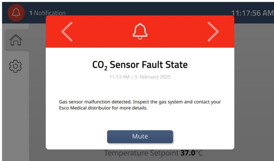
Figure 15.22 CO<sub>2</sub> sensor fault state alarm on the docking station display
