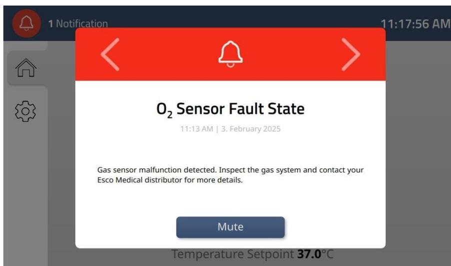
Figure 15.23 O<sub>2</sub> sensor fault state alarm on the docking station display
