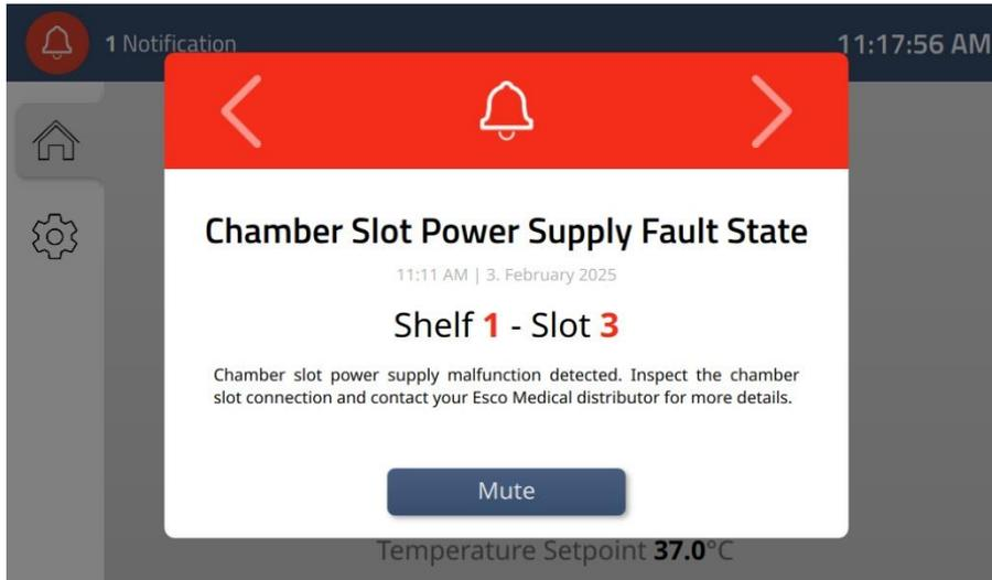
**Figure 15.27** Chamber slot power supply fault state alarm
