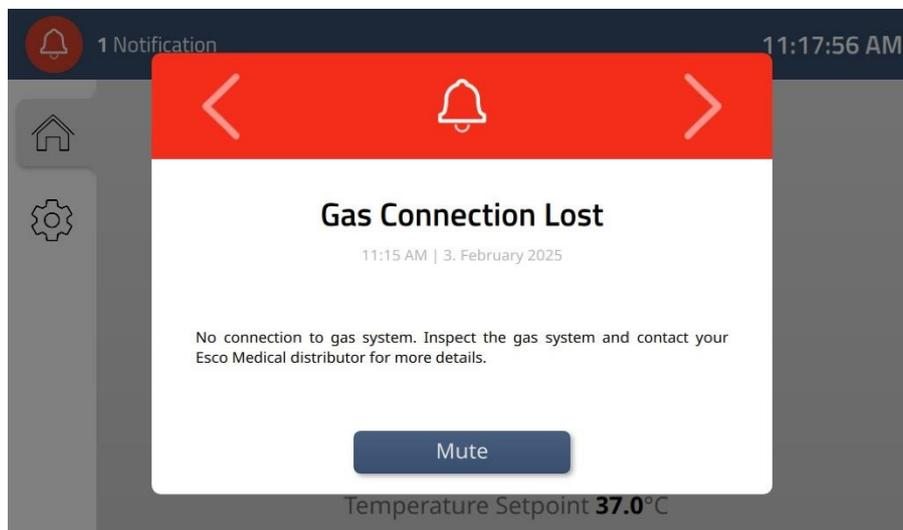
Figure 15.24 Gas connection lost alarm on the docking station display
