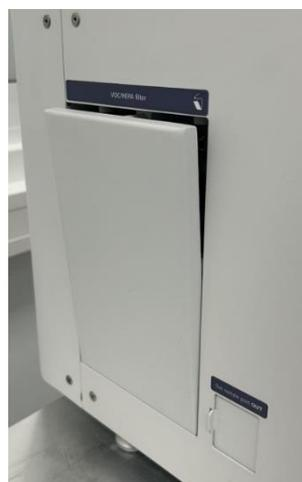
**Figure 12.1** The push-to-open hatch
