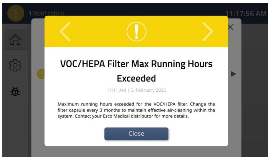
Figure 15.50 VOC/HEPA filter running hours exceeded warning
