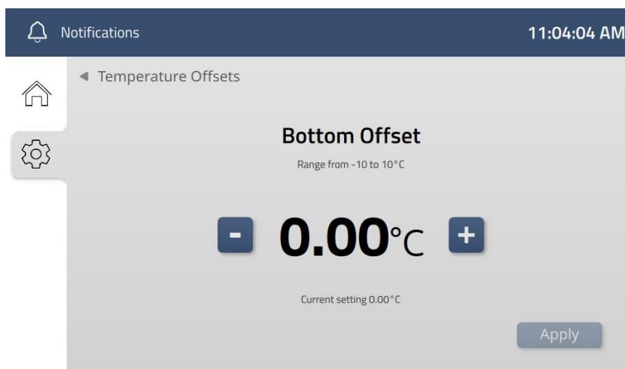
Figure 14.10 Bottom temperature offset
