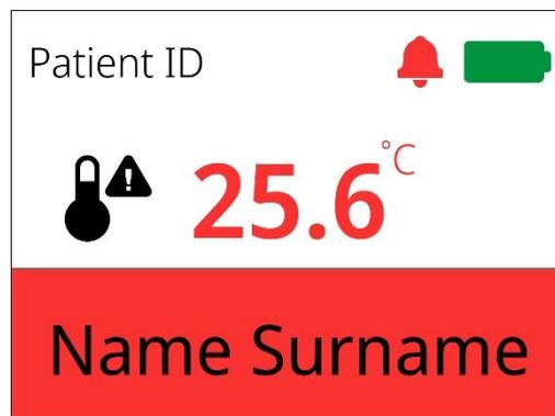
**Figure 15.9** Low-temperature alarm indication on the undocked chamber's display
