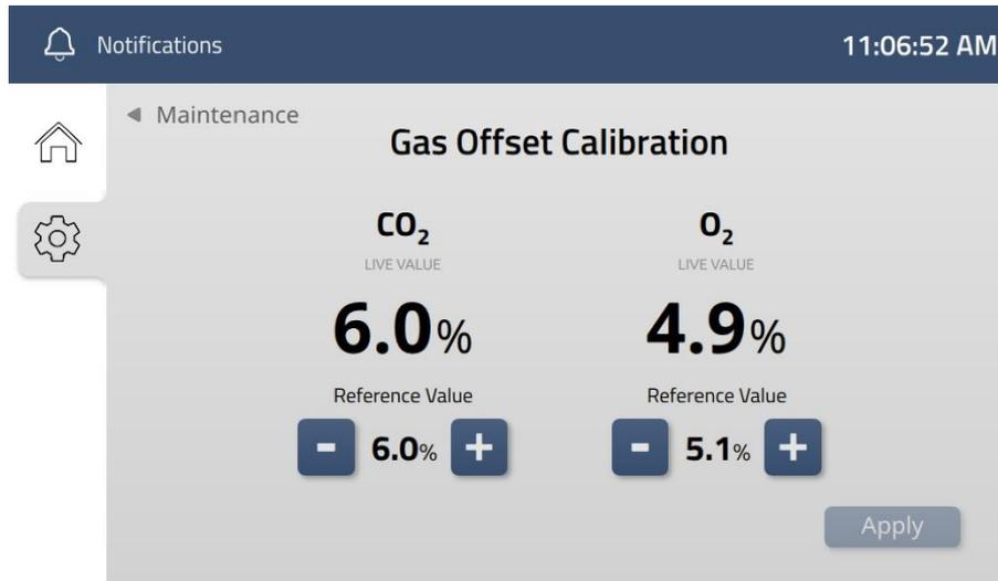
Figure 14.26 Gas offset being calibrated
