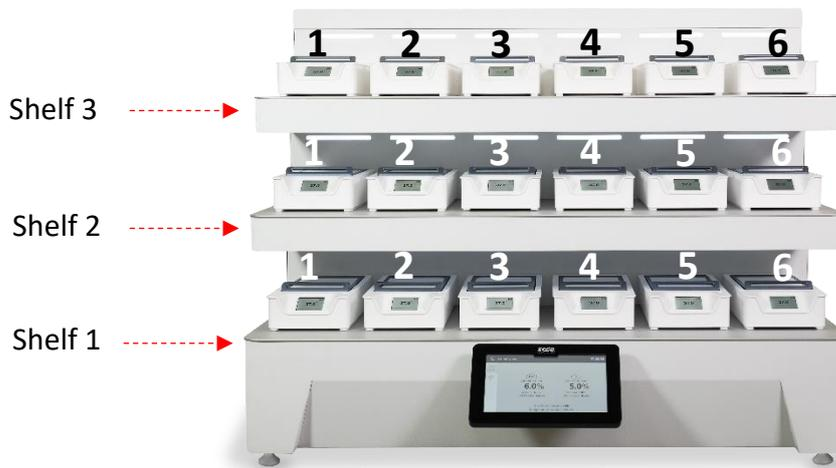
**Figure 7.1** MIRI® M multiroom IVF incubator docking position numbers and shelf names
