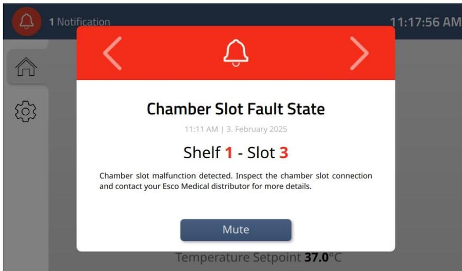
**Figure 15.26** Chamber slot fault state alarm
