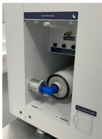
**Figure 12.3** Filter's elbow blue fitting inserted
