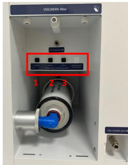
Figure 22.1 Connections of PT-1000 Class B sensors
