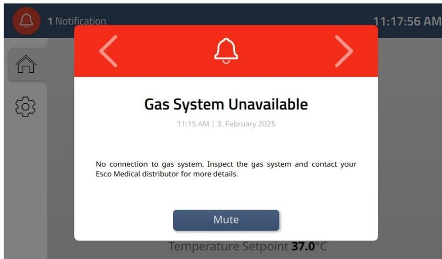
**Figure 15.25** Gas system unavailable alarm on the docking station display
