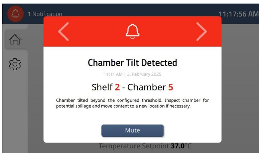
**Figure 15.33** Chamber tilt alarm indication on the docking station's display panel
