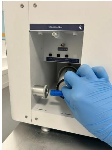
Figure 12.6 Filter's blue elbow fitting pushed out
