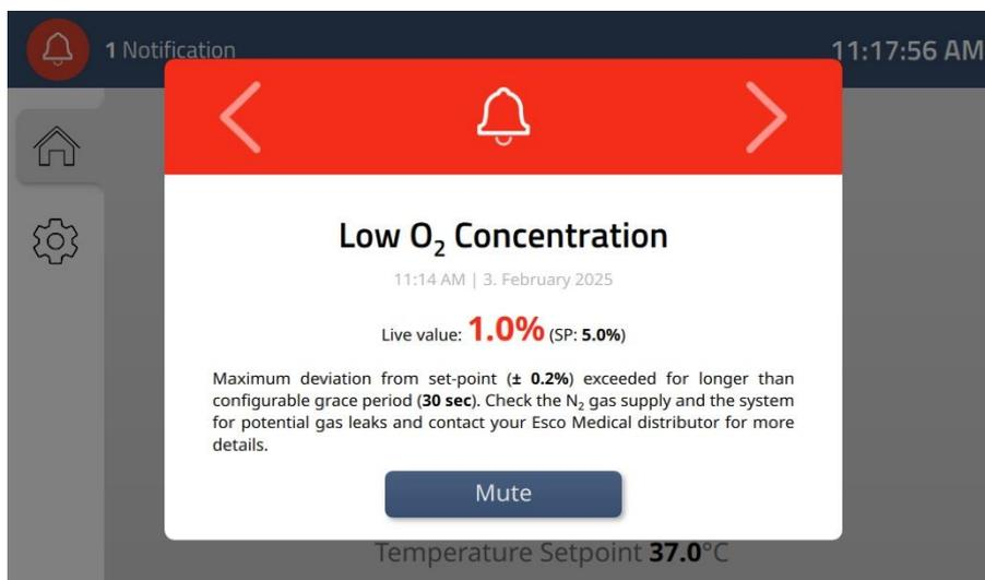
Figure 15.15 Low O<sub>2</sub> concentration alarm indication on the docking station's display panel
