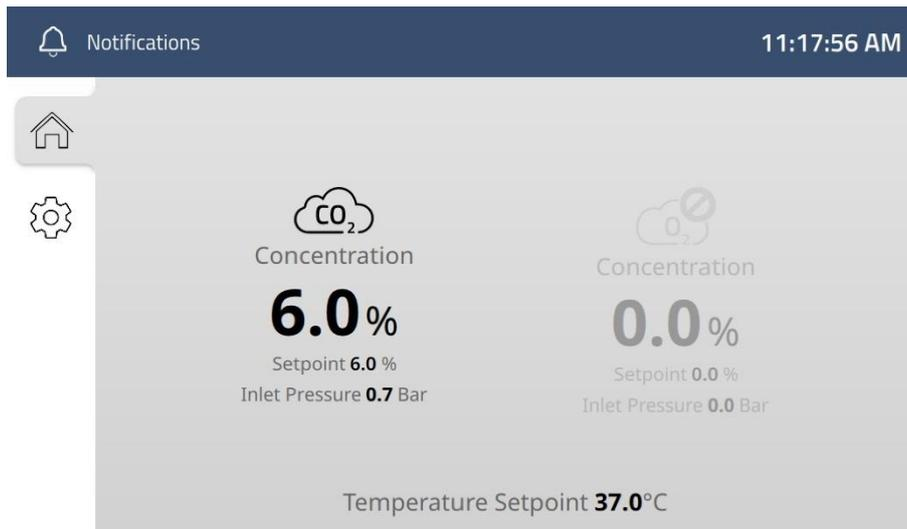
Figure 14.13 Main page with O<sub>2</sub> regulation turned off
