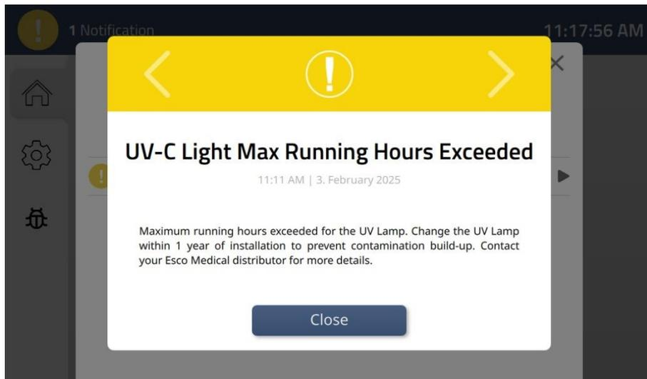
Figure 15.49 UV-C light running hours exceeded warning
