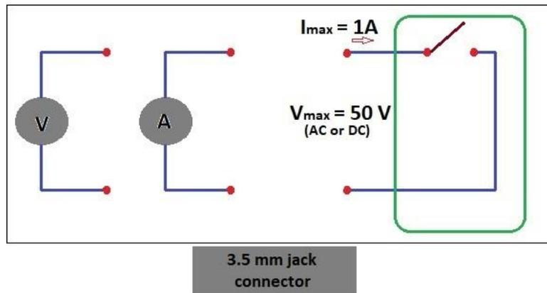
Figure 24.2 "Open circuit" alarm mode
