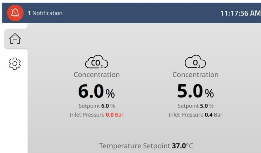
**Figure 15.18** A muted CO<sub>2</sub> gas pressure alarm view on the main display
