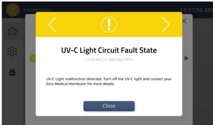
Figure 15.48 UV-C light circuit fault state warning
