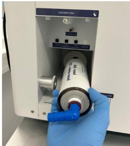
Figure 12.7 Filter push out of the device
