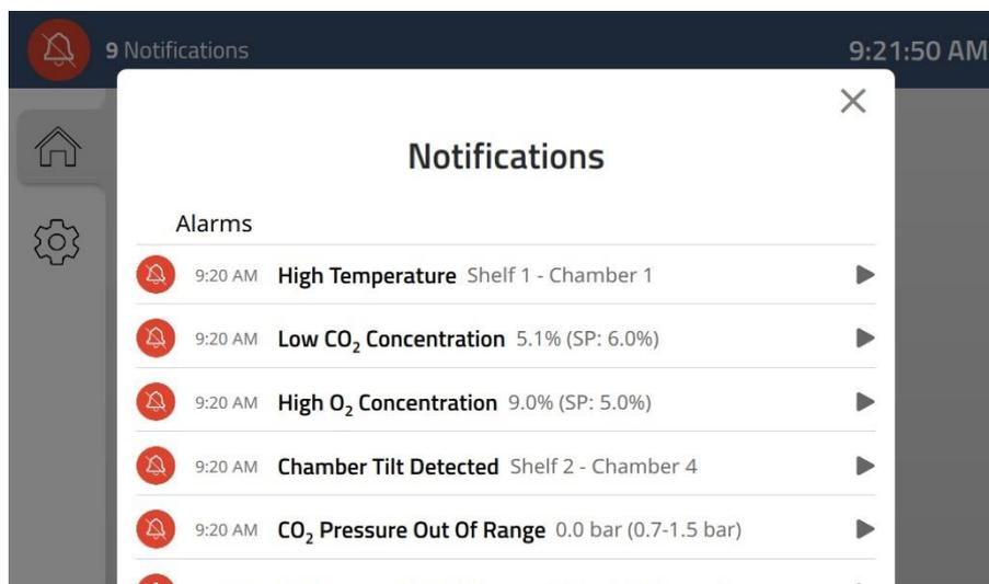
Figure 15.37 Notifications log showing multiple alarms
