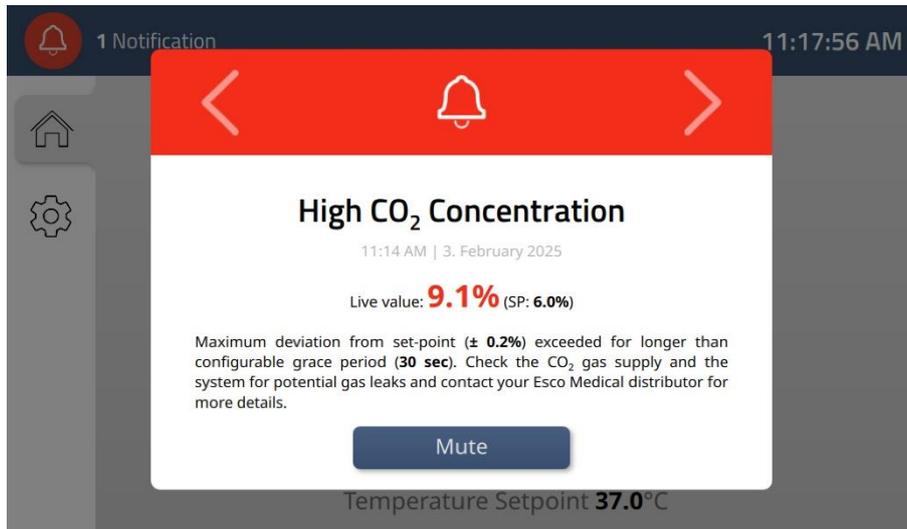
**Figure 15.11** High CO<sub>2</sub> concentration alarm indication on the docking station's display panel
