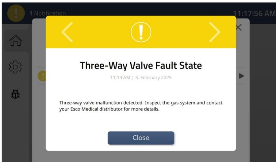
**Figure 15.53** Three-way valve fault state warning
