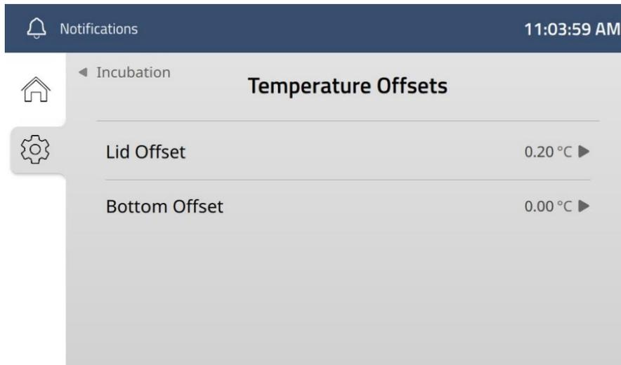
Figure 14.8 Temperature Offset settings
