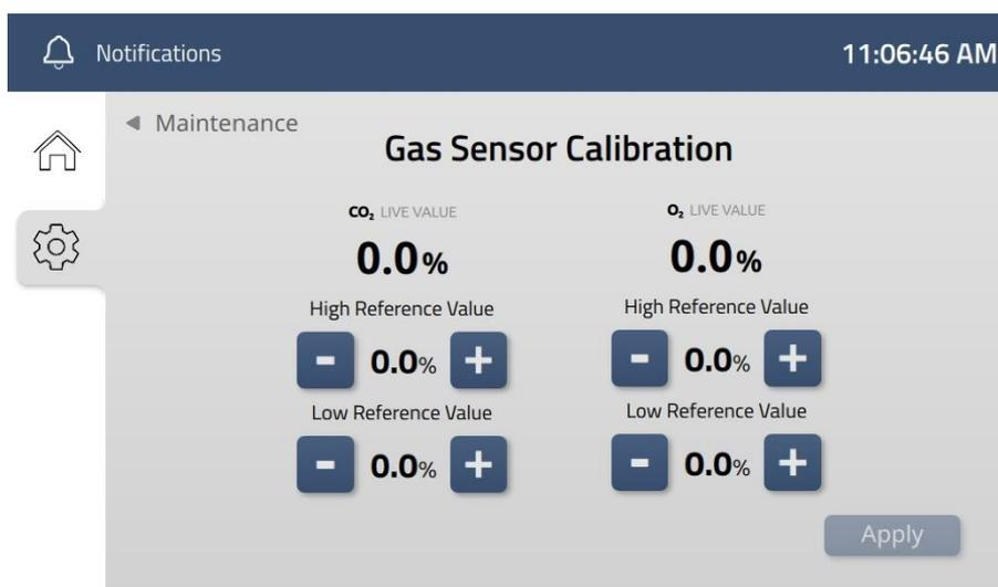
Figure 14.24 High reference value for CO<sub>2</sub> being calibrated
