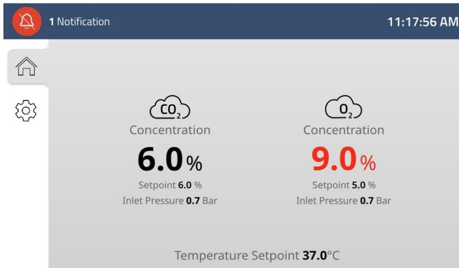
Figure 15.16 A muted O<sub>2</sub> concentration alarm on the main display
