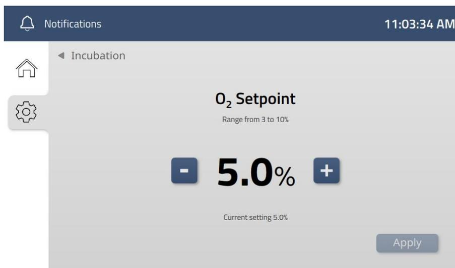
Figure 14.7 O<sub>2</sub> Setpoint view
