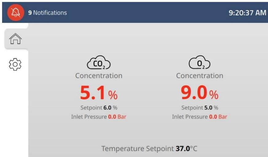
Figure 15.36 Multiple alarms in the main display
