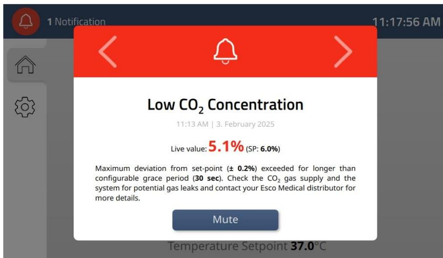
**Figure 15.12** Low CO<sub>2</sub> concentration alarm indication on the docking station's display panel
