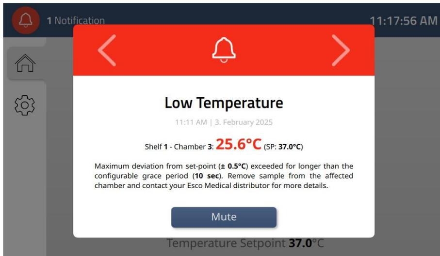
**Figure 15.1** The alarm indication on the docking station display with a mute option
