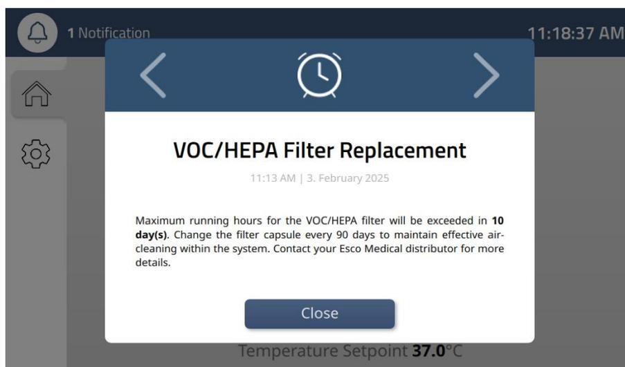
Figure 14.21 The VOC/HEPA filter reminder
