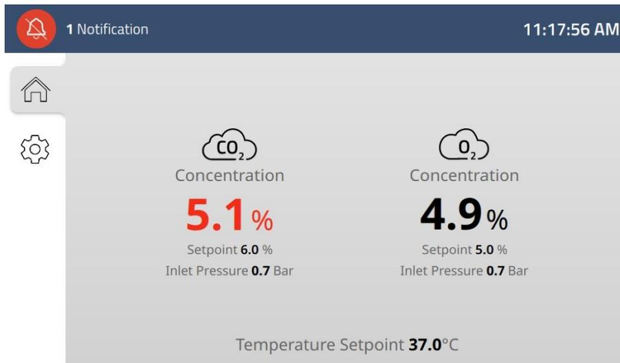
Figure 15.13 A muted CO<sub>2</sub> concentration alarm on the main display
