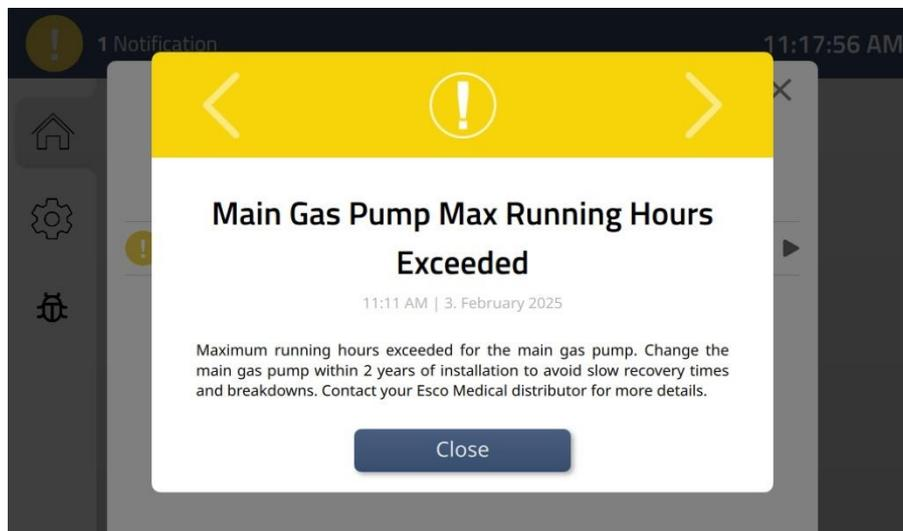
Figure 15.51 Main gas pump running hours exceeded warning
