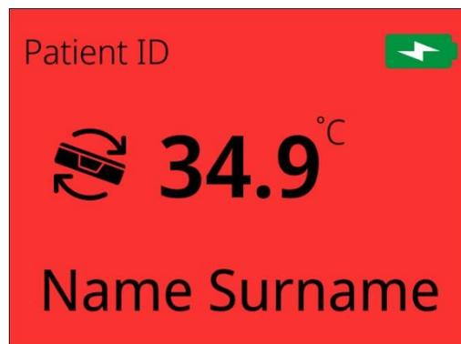
**Figure 15.39** Multiple alarm indication on the undocked chamber’s display (tilt/temperature alarms active)
