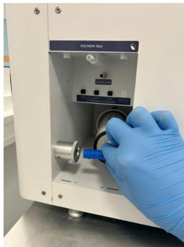
**Figure 12.2** Filter's straight blue fitting inserted
