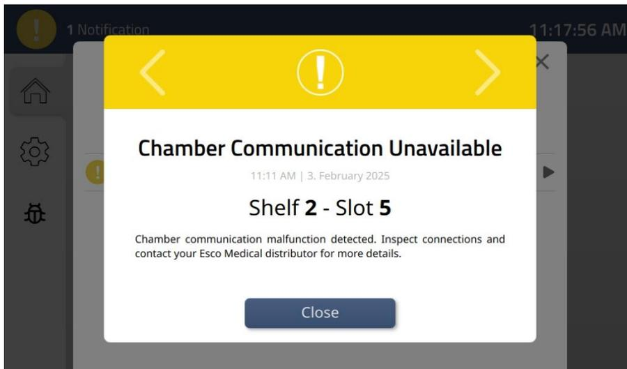
**Figure 15.55** Chamber communication unavailable warning
