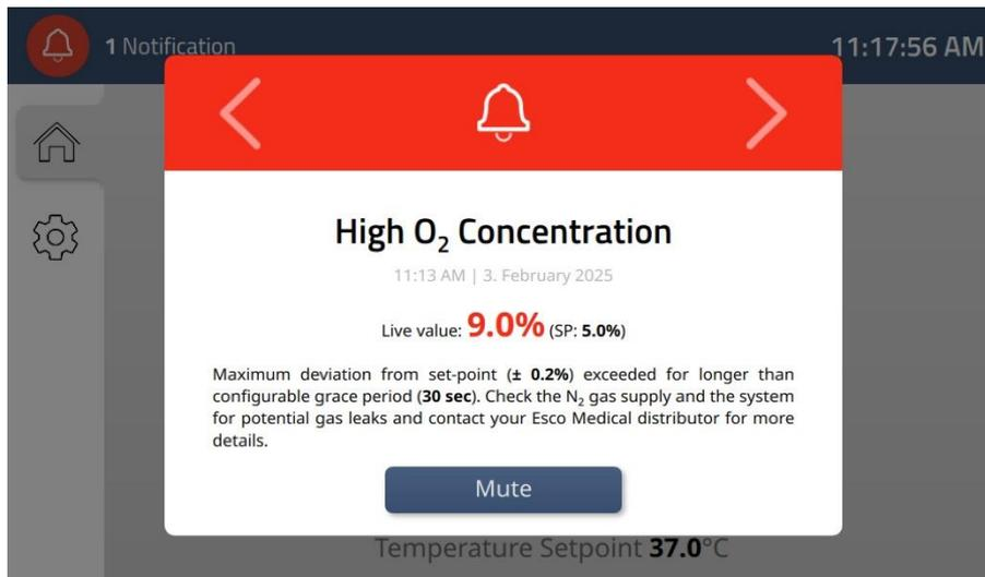
Figure 15.14 High O<sub>2</sub> concentration alarm indication on the docking station's display panel
