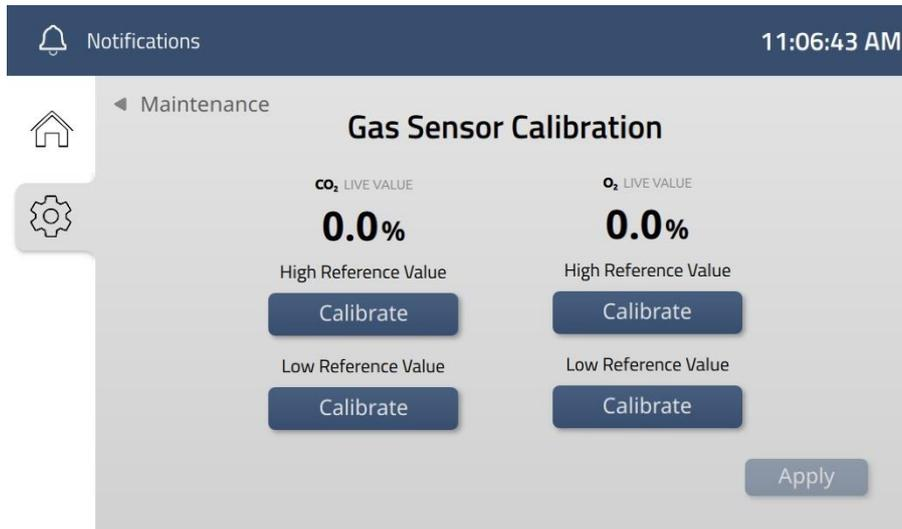
Figure 14.23 Gas sensor calibration page
