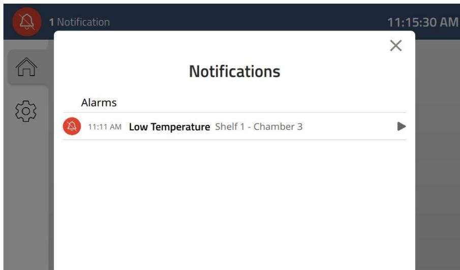
Figure 15.5 The notification log with a muted alarm
