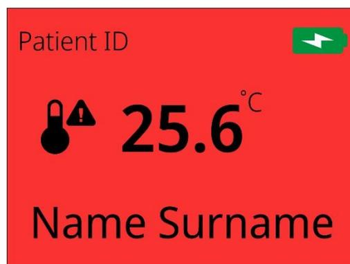
**Figure 15.2** The alarm indication on the display of a docked chamber
