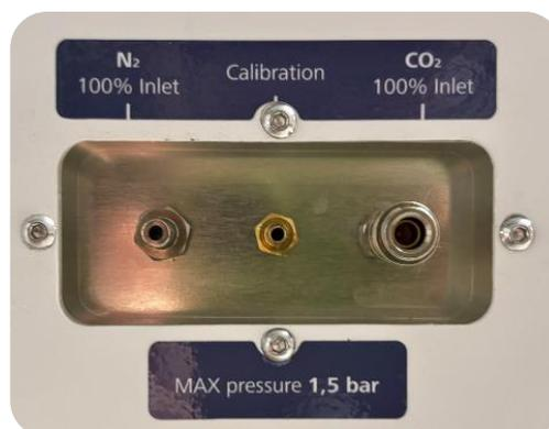
**Figure 11.1** Gas inlets on the back of the MIRI<sup>®</sup> M multiroom IVF incubator
