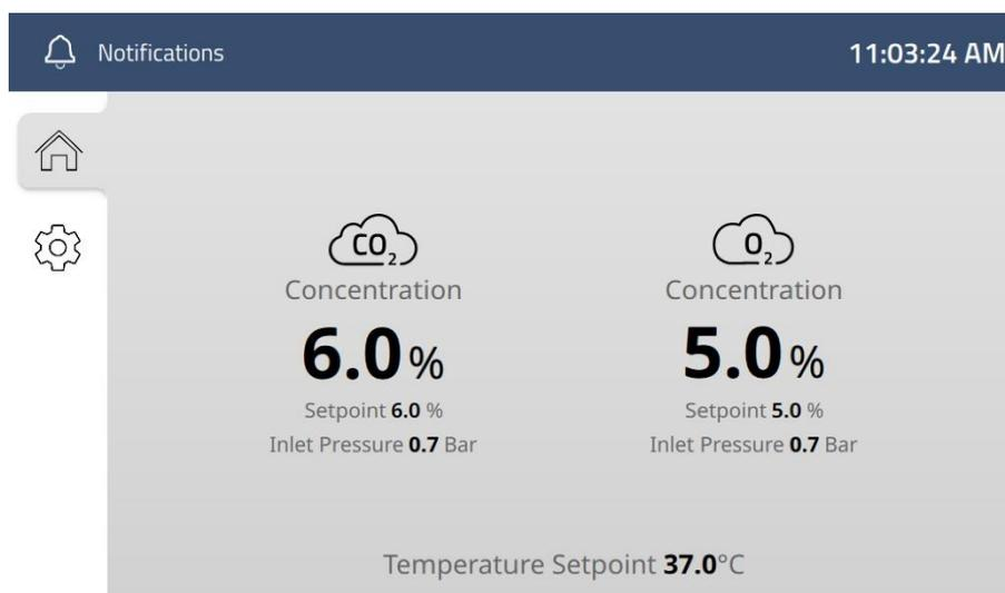
Figure 14.2 MIRI<sup>®</sup> M incubator main display view
