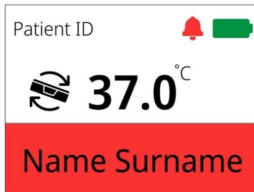
Figure 15.31 Tilt alarm indication on an undocked chamber's display
