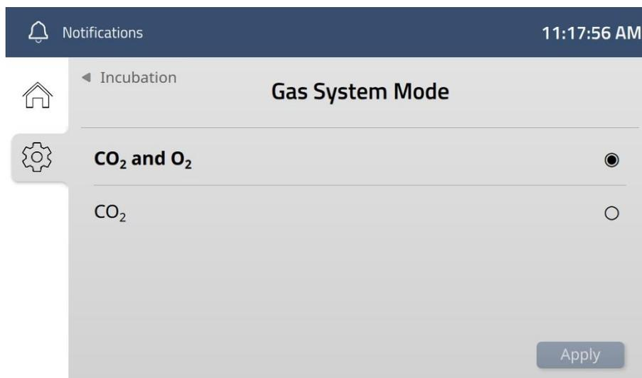
**Figure 14.12** Gas system mode settings
