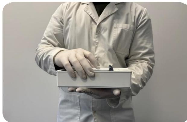
**Figure 14.35** Correct chamber carrying procedure
