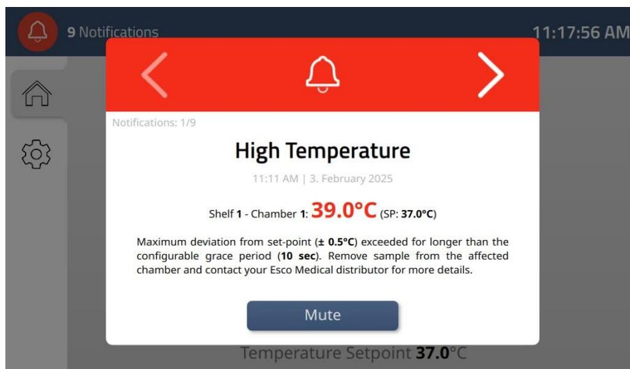
**Figure 15.35** Multiple alarm indication on the docking station's display panel
