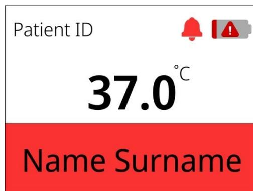
Figure 15.29 Critically low battery alarm
