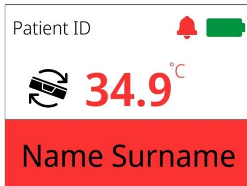
**Figure 15.38** Multiple alarm indication on the undocked chamber’s display (tilt/temperature alarms active)
