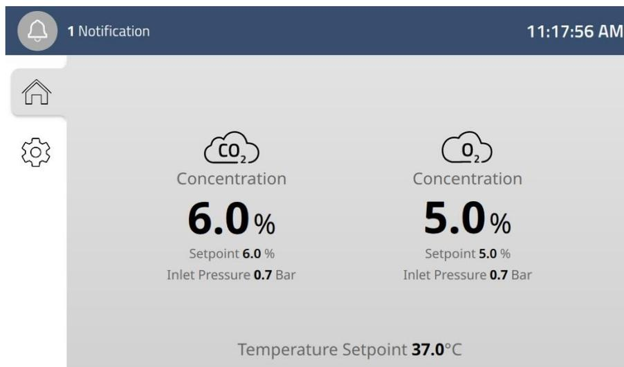
Figure 15.41 The unacknowledged alarm indication on the main display
