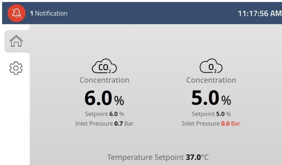
Figure 15.20 A muted N<sub>2</sub> gas pressure alarm view on the main display panel
