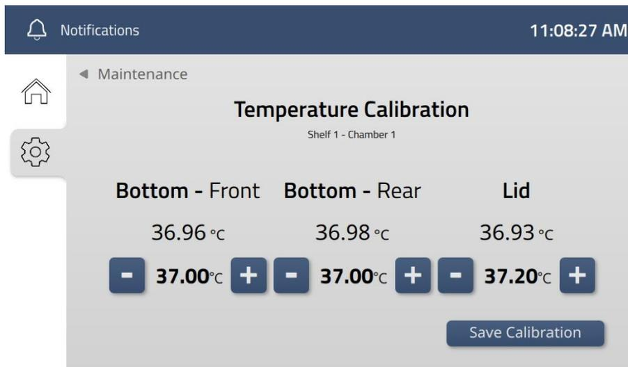
Figure 14.29 Temperature calibration page with calibrated values
