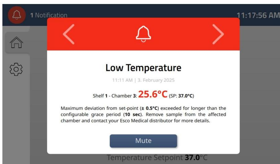
**Figure 15.7** Low-temperature alarm indication on the docking station's display panel
