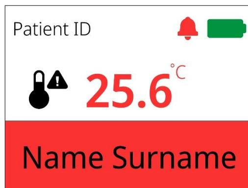
**Figure 15.3** Example of the alarm indication on an undocked Chamber
