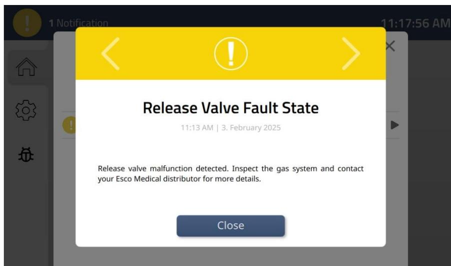
**Figure 15.54** Release valve fault state warning
