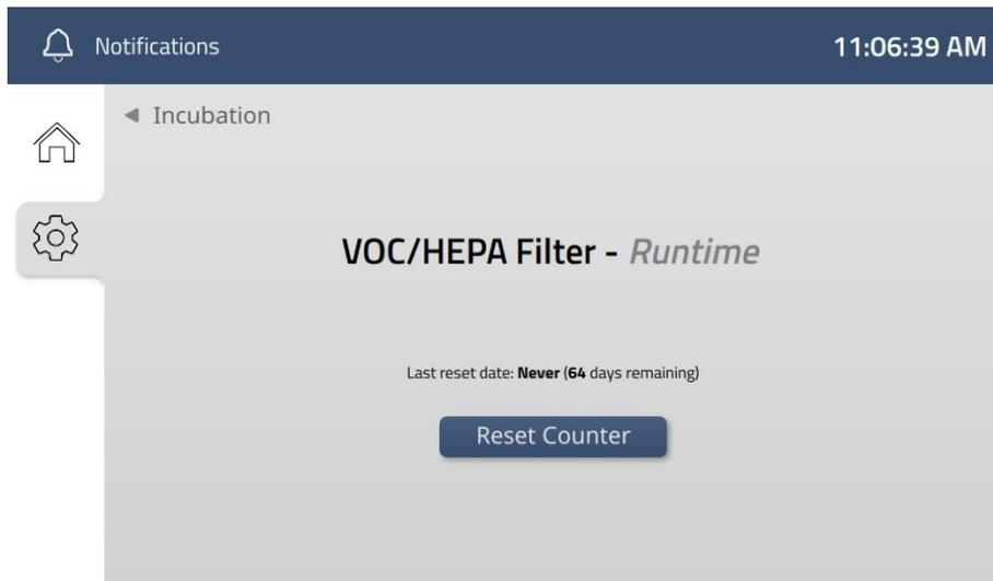
Figure 14.22 The VOC/HEPA filter runtime reset button
