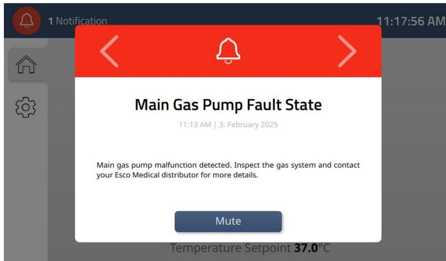
**Figure 15.21** Gas Pump fault state alarm indication on the docking station's display panel
