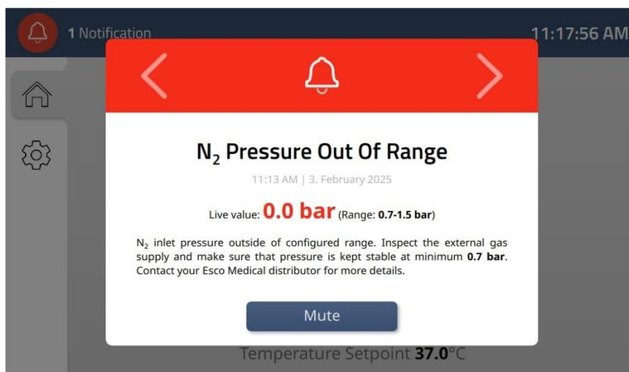
**Figure 15.19** N<sub>2</sub> pressure out-of-range alarm indication on the docking station's display panel
